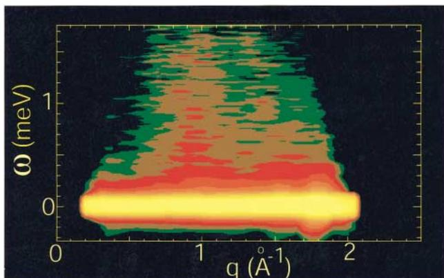
FIG. 1 (color). A contour plot of  $\chi''(q, \omega)$  of  $\text{UCu}_4\text{Pd}$  at 1.6 K.
